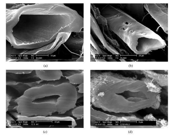
FIGURE 1. Scanning electron micrographs of TMP lumens fiber (a), TMP pits fiber (b), mixed tropical lumens fiber (c) (Ainun 2006) and efb lumens fiber (d) (Humaizah 2002)
