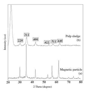
FIGURE 3. X-Ray diffractograms of magnetic particle  $Fe_{3}O_{4}$  (a) from pulp sludge (b) for IS6
